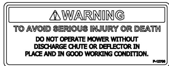
P-12706... WARNING – Deck Discharge Opening Safety.
