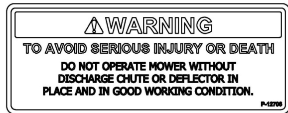
P-12706... WARNING – Deck Discharge Opening Safety.
