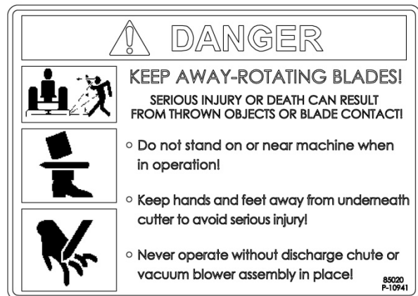
P-10941... DANGER – Rotating Blade Safety.
