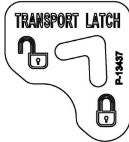
P-13437... Transport Latch – Lock position will permit the deck to lock in transport when raised to that position. Un-lock position will not lock the deck in transport when raised in transport.
