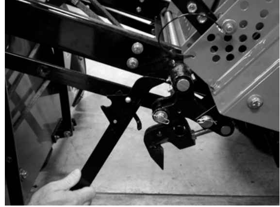
Deck Prop being placed against the Deck lift casting.
