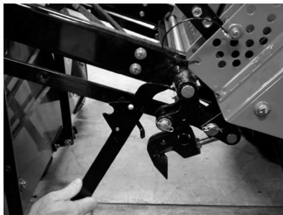
Deck Prop being placed against the Deck lift casting.
