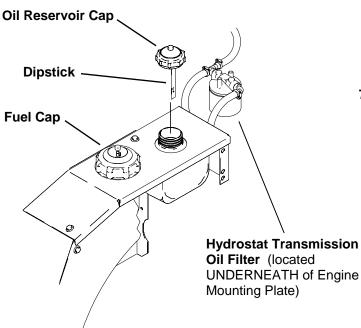
Check the oil level in hydrostatic transmission oil reservoir after every 25 hours of usage. Clean the oil reservoir cap and the area around it prior to removal. Check the oil level on the dipstick. The proper oil level should register between the marked hole on the dipstick and the end of the dipstick. Replenish as needed with 20W-50 Motor Oil. **DO NOT OVER FILL.** When checking the oil level, be very careful to keep the reservoir clean
